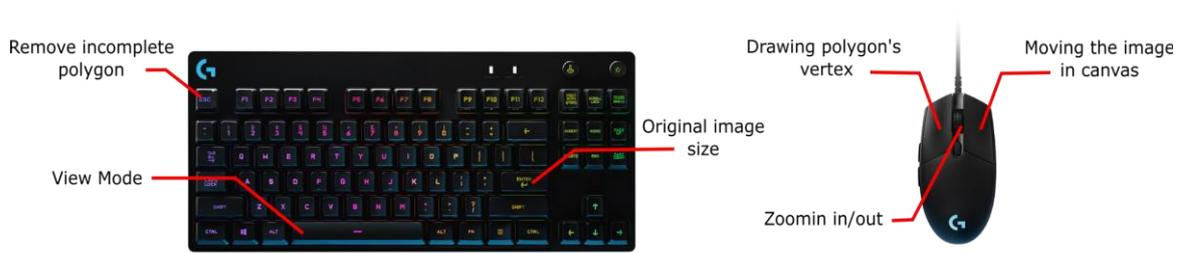
**Fig. 3.5.** Mouse and keyboards operational keys and their function
